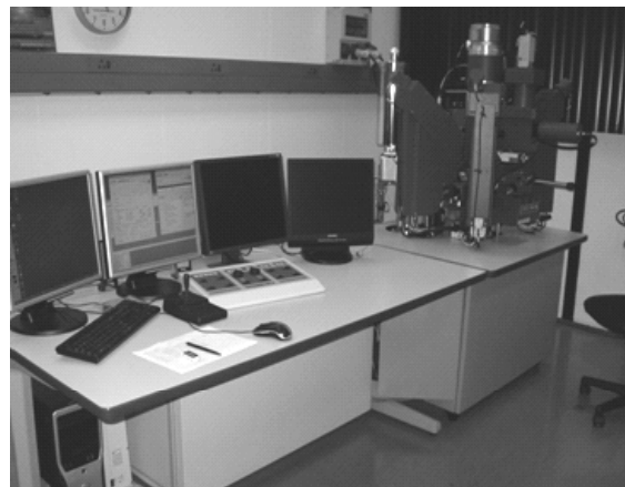
Figure 7: The Cameca SX-100 electron microprobe at the University of Johannesburg. This instrument is being used to determine small amounts of dissolved base metals in slag samples from the six-in-line furnaces and the slag-cleaning furnace.
