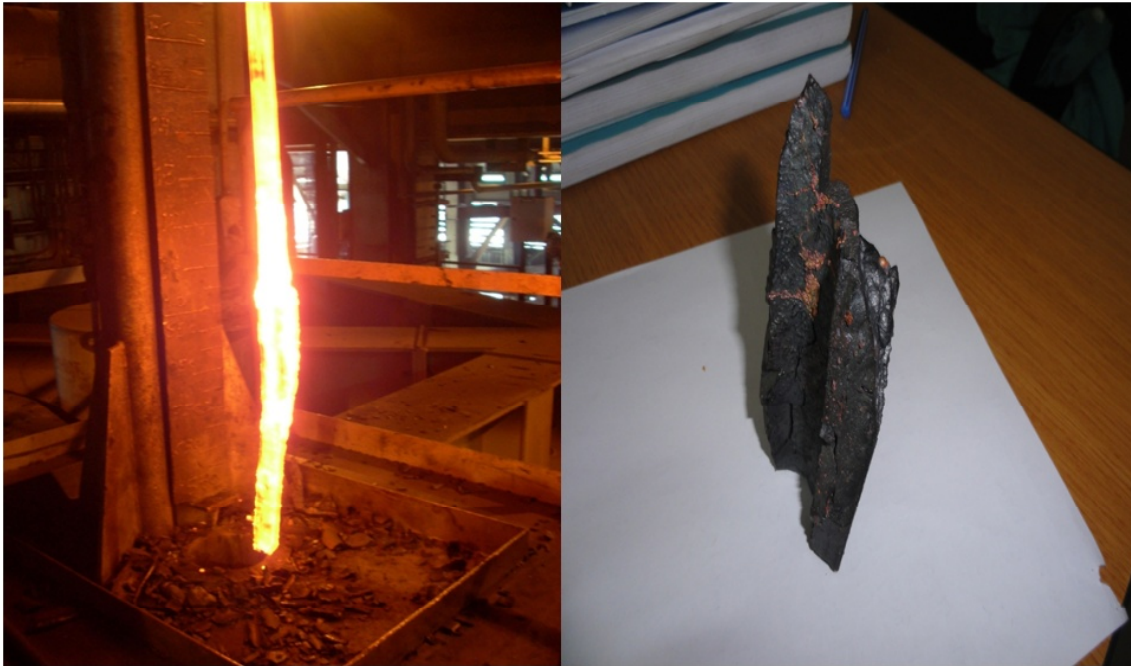
Figure 4: Intermediate phase formation and entrainment of copper droplets
