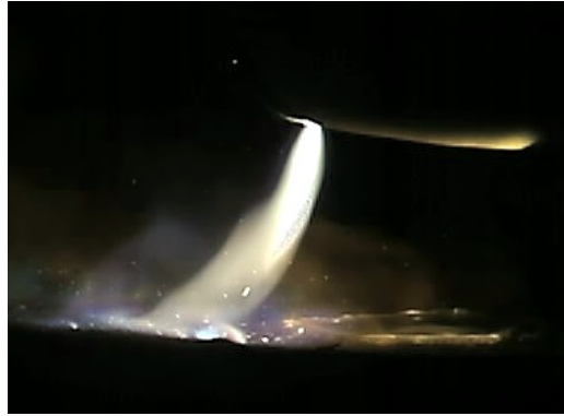
Figure 4: Reverse polarity (anode electrode) arc, 1kA, ~110V, 5cm length
