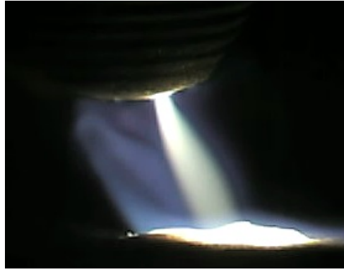
Figure 3: Traditional polarity (cathode electrode) arc, 1kA, ~80V, 5cm length
