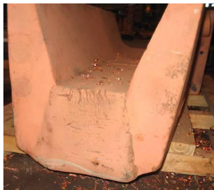
Figure 6: Repaired launder tip that originally had the rounded launder edge
