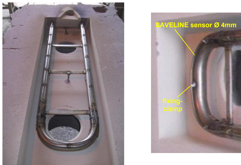
Figure 8: Prepared metal tube inside the sand mould
