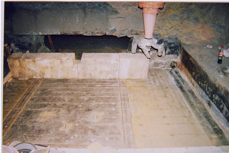
Figure 5: SAVELINE sensors applied in the condenser floor of an Imperial Smelter
