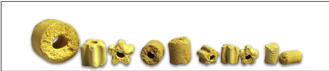
Figure 1: Photograph of catalyst pieces, courtesy Haldor Topsøe A/S http://www.haldortopsøe.com The outside diameter of the largest piece (far left) is 20 mm.
