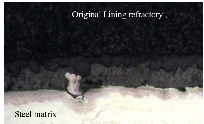
(b) The iron drops start to detach from the iron phase
