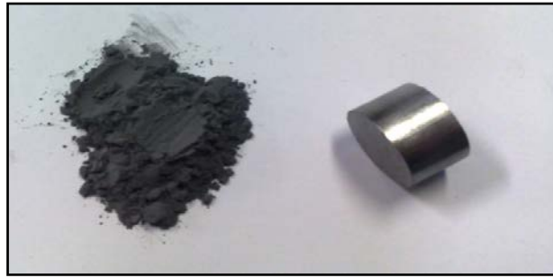
Fig. 1 Carbonyl iron powder and pressed sample
