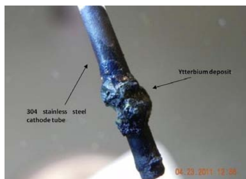
Figure 12. Yb metal deposit on the stainless steel cathode
