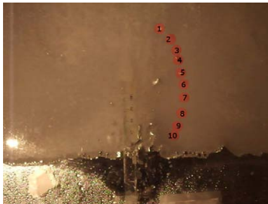
Fig. 4 The trajectory of a droplet falling back to the metal
