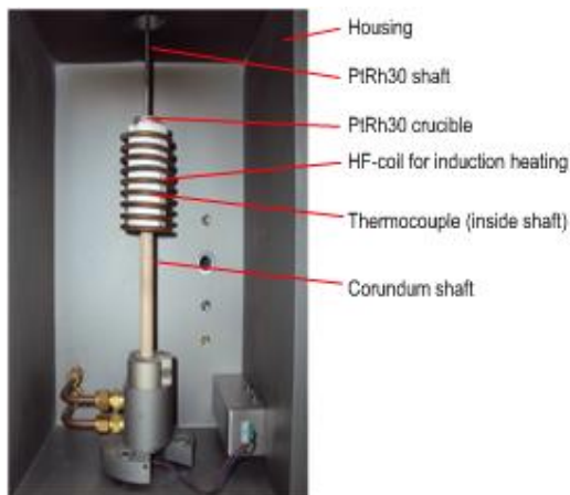
Fig. 1: Detail of measurement chamber of the viscometer (Bähr Thermoanalyse GmbH)
