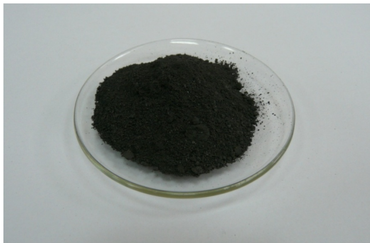
Fig 10. Obtained dusts containing more than 76 wt-% Te.
