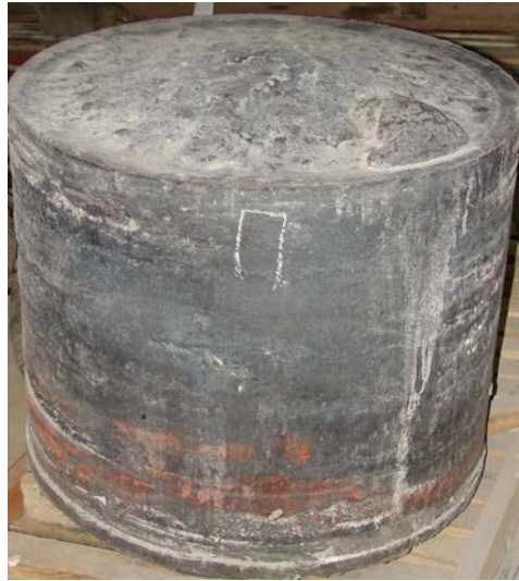
Fig. 2 The view of surface of 920 mm diameter ingot.
