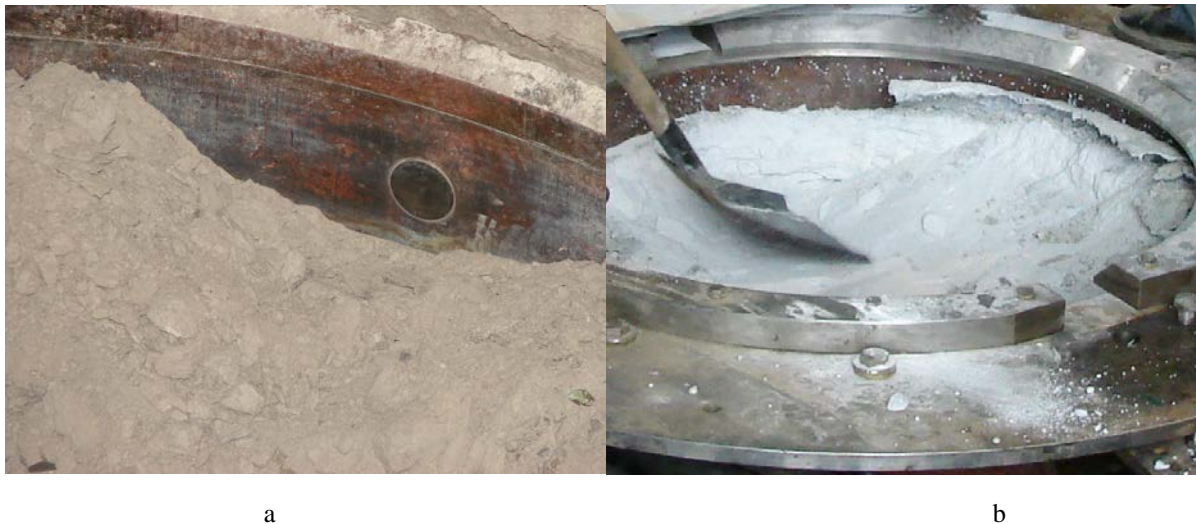
Fig.1 The view of slag bath in the mold of the 920 mm diameter after cooling (a) without metal remelting and after ingot melting (b).
