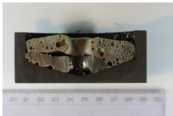
Figure 3 Cross section of the crucible after the smelting test
