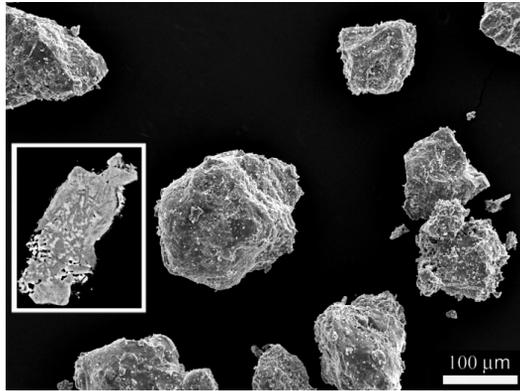
Figure 4: SEM secondary electron image showing the NIC sample after reaction in EDAMM for 10 minutes under Ar gas. The scale bar is 100  $\mu\text{m}$
