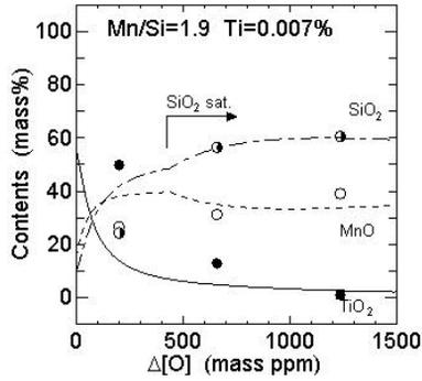
Figure 7: Comparison between calculated composition change of scum and experimental one in the case of steel with titanium
