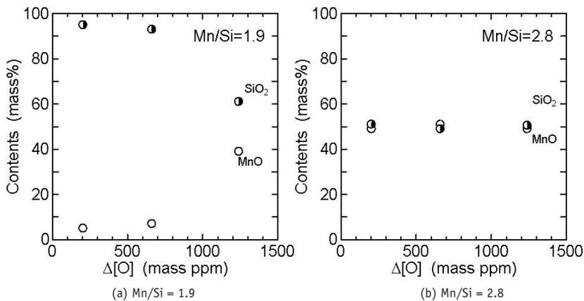
Figure 4: Composition changes in scum during Ar+O<sub>2</sub> gas blowing. (a) Mn/Si = 1.9 and (b) Mn/Si = 2.8
