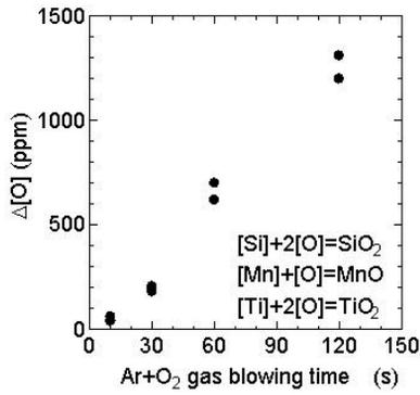
Figure 2: Relationship between  $\Delta[O]$  and Ar+O<sub>2</sub> gas blowing time
