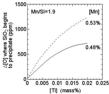
Figure 8: Influence of [Ti] content on minimum  $\Delta O$  for solid  $\text{SiO}_2$  precipitation in scum
