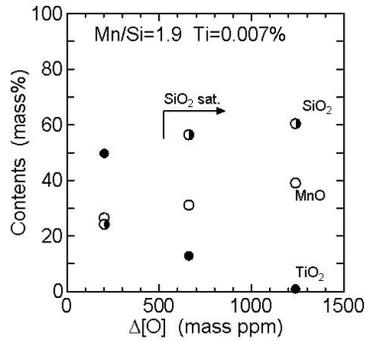
Figure 5: Composition Changes in Scum during Ar+O<sub>2</sub> Gas Blowing onto steel with 0.007%Ti
