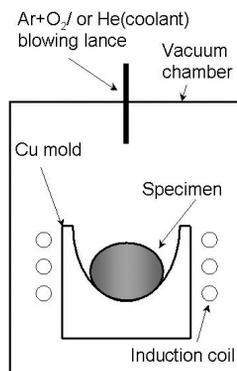
Figure 1: Experimental apparatus for reoxidation of steels
