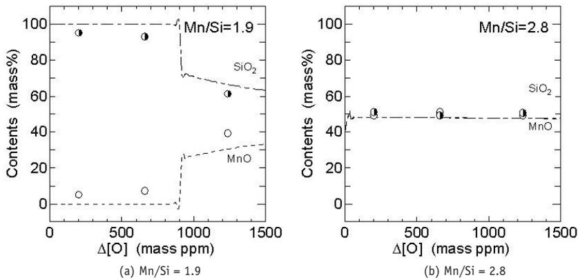
Figure 6: Comparison between calculated composition change of scum and experimental one in the case of steel without titanium. (a) Mn/Si = 1.9 and (b) Mn/Si = 2.8
