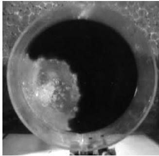
Figure 2: Photo of plume eye taken from top. Water (light area)-silicone oil (dark area) system 1 lpm in the first plug and zero in the system: 10. Other (1-0), 2 cm layer of oil of 50 cSt.
