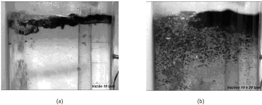
Figure 12: (a) Emulsification of kerosene for flow rate of 10 lpm, one plug ;
