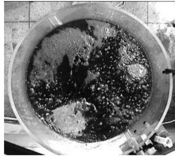
Figure 3: Photo of plume eye taken from top. Water/ZnCl<sub>2</sub> solution (light area)-silicone (dark area) air flowrate lpm in the first plug and 5 lpm in the other (10 - 5), 3 cm layer of oil of 500 cSt.
