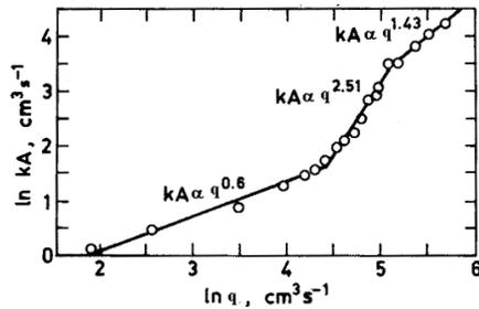
Figure 10: Apparent mass transfer coefficient for ladle desulfurization as a function of gas flowrate [1]
