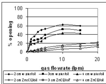
Figure 6: Comparison between eye opening in the systems water\_ZnCl<sub>2</sub> and water / 50 cSt oil as function of gas flowrate and slag tickness
