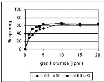
Figure 4: Relationship between % opening and gas flowrate for viscosities of 50 cSt and 500 cSt, and oil layer thickness of 2 cm.
