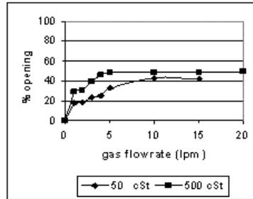
Figure 5: Relationship between % opening and gas flowrate for viscosities of 50 cSt and cSt, and oil layer thickness of 4 cm.
