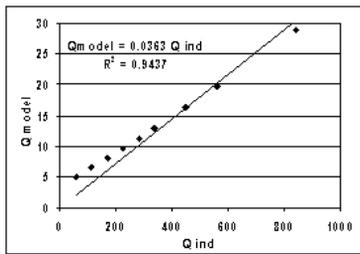
Figure 8: Flow rates (STP lpm) in the model and industrial machine, capable of producing the same % opening
