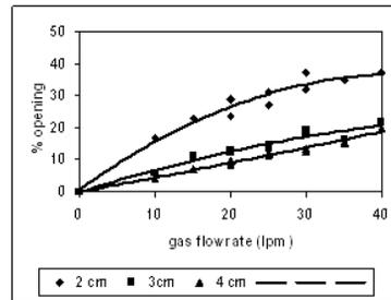
Figure 7: % opening vs flowrate for water\_ZnCl<sub>2</sub> / 500 cSt oil system
