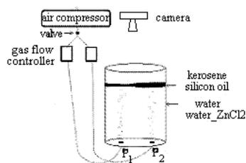
Figure 1: Schematic of the physical model of the ladle
