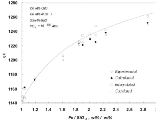
Figure 5: Calculated and experimental spinel liquidus line (open - experimental; closed - interpolated points; circles - variable CaO, MgO and Al<sub>2</sub>O<sub>3</sub> concentrations; and square - interpolated points with CaO = 2.0 wt%, MgO = 0.5 wt% and Al<sub>2</sub>O<sub>3</sub> = 4.0 wt%) at PO<sub>2</sub> = 10<sup>-8.5</sup> atm
