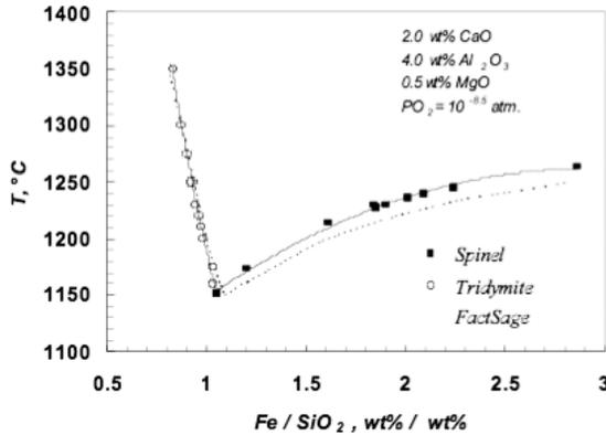
Figure 6: Liquidus trydymite and spinel line for the “Cu<sub>2</sub>O-FeO-Fe<sub>2</sub>O<sub>3</sub>-SiO<sub>2</sub>-CaO-MgO-Al<sub>2</sub>O<sub>3</sub>” slag system in the range of compositions and temperatures directly relevant to electric furnace practice and  $P_{O_2} = 10^{-8.5}$  atm
