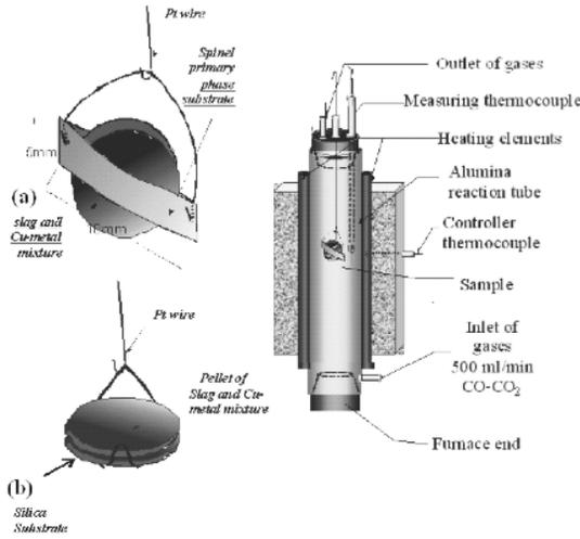
Figure 2: Schematic experimental apparatus with substrates of (a) spinel and (b) silica
