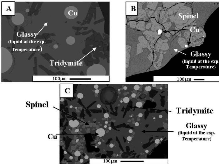
Figure 3: SEM of liquid slag in equilibrium with tridymite or/and spinel at the condition of copper sat. (A:Tridymite sat. 1250°C, B:Spinel sat. 1235°C, C:Tridymite and spinel sat. 1150°C)
