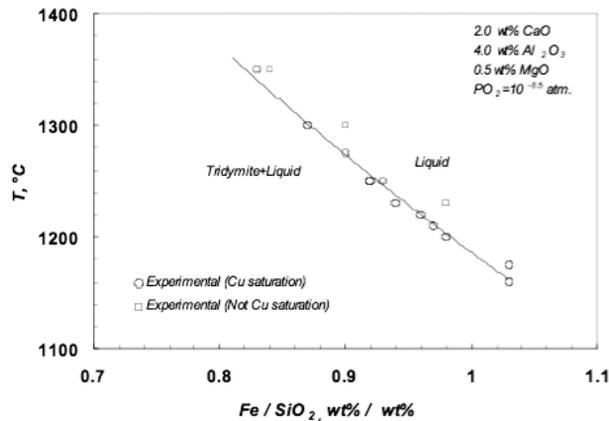
Figure 4: Measured tridymite liquidus line (open marks–Cu sat.; closed marks–Not Cu sat.) for a slag with CaO = 2.0 wt%, MgO = 0.5 wt% and Al<sub>2</sub>O<sub>3</sub> = 4.0 wt% at P<sub>O<sub>2</sub></sub> = 10<sup>-8.5</sup> atm
