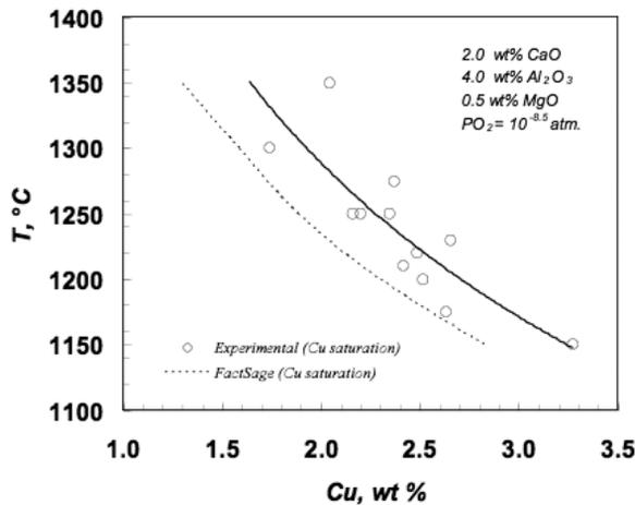
Figure 7: Copper solubility in slag as a function of temperature along the tridymite liquidus at metallic copper saturation for the electric furnace practice (solid line experimental trend) and  $P_{O_2} = 10^{-8.5}$  atm
