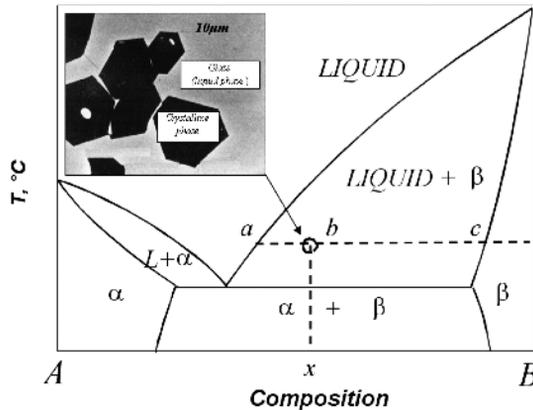
Figure 1: Schematic of approach to phase equilibrium determination using sub-liquidus equilibration, quenching and EPMA
