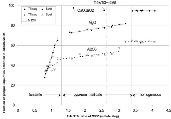
Figure 3: Partition of gangue impurities between  $\text{M}_3\text{O}_5$  and glassy silicate phase
