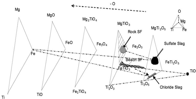
Figure 1: Stoichiometric relationship between ilmenite feed and smelting products
