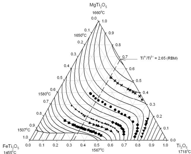
Figure 2: Liquidus isotherms in  $\text{FeTi}_2\text{O}_5$ - $\text{MgTi}_2\text{O}_5$ - $\text{Ti}_3\text{O}_5$  system
