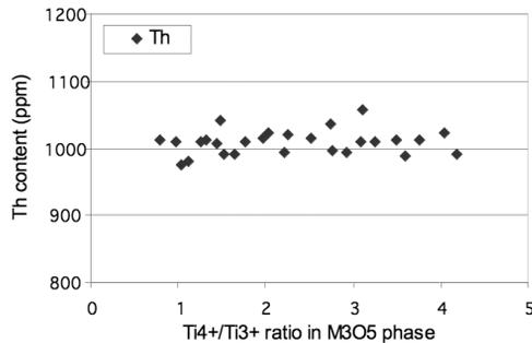
Figure 5: Th content in  $\text{M}_3\text{O}_5$  phase saturated with  $\text{ThTi}_2\text{O}_6$
