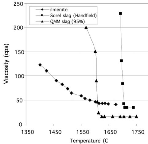
Figure 7: Viscosity of ilmenite and QMM slag
