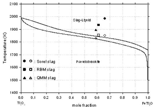
Figure 6:  $\text{FeTi}_2\text{O}_5$ - $\text{Ti}_3\text{O}_5$  system with melting point measurements
