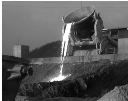
Figure 2: The air-cooling process for metallurgical slags
