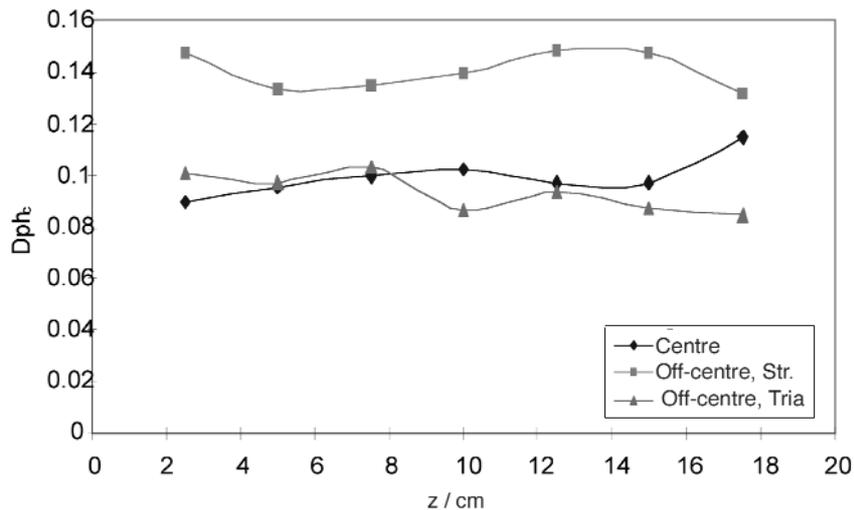
Figure 3. Axial variation of the dispersed phase holdup for different configuration at 0.01081 m<sup>3</sup>/s
