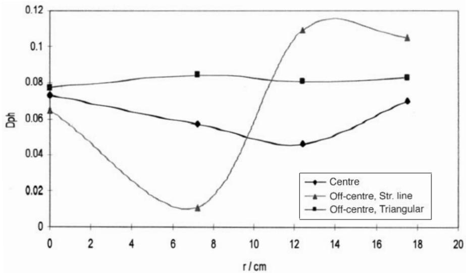
Figure 6. Effect of tuyere configuration on the radial variation of the Dph on the left-axis of the tank ( $0.00599 \text{ m}^3/\text{s}$  and  $z = 15 \text{ cm}$ )
