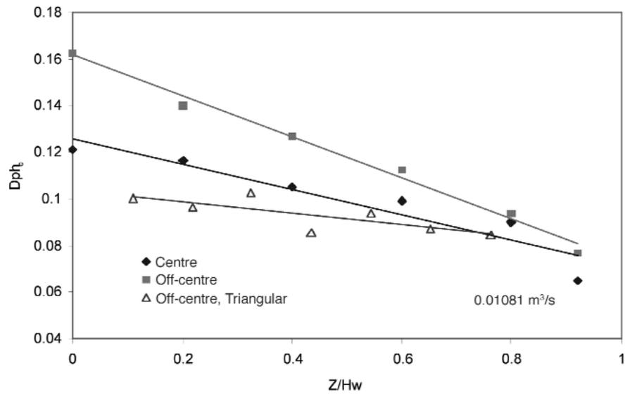
Figure 10. Effect of tuylene configuration on the dispersed phase holdup along the centreline
