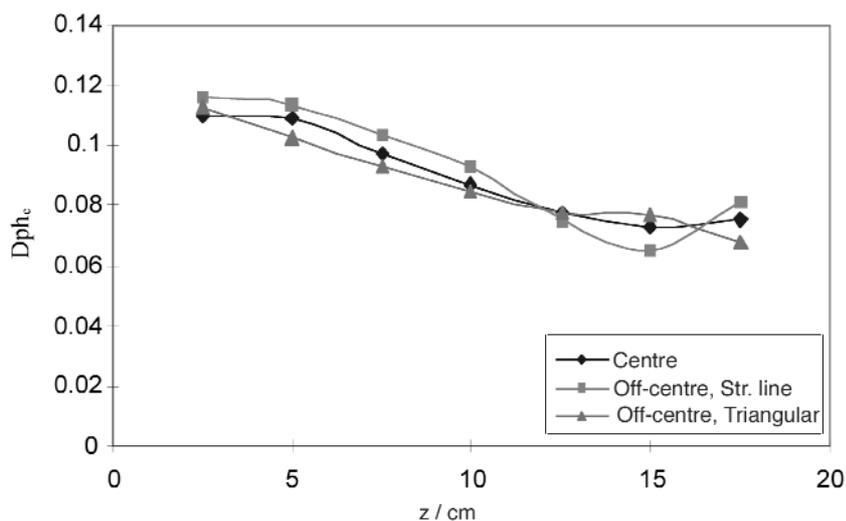
Figure 2. Axial variation of the dispersed phase holdup for different configuration at 0.00599 m<sup>3</sup>/s
