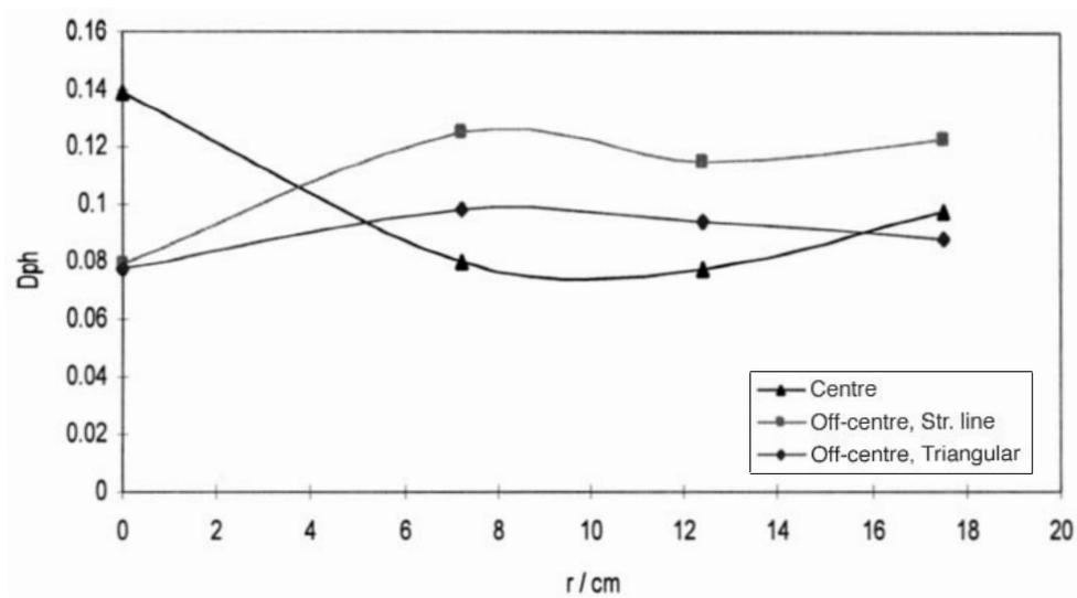
Figure 7. Effect of tuyere configuration on the radial variation of the Dph on the left-axis of the tank ( $0.00849 \text{ m}^3/\text{s}$  and  $z = 15 \text{ cm}$ )
