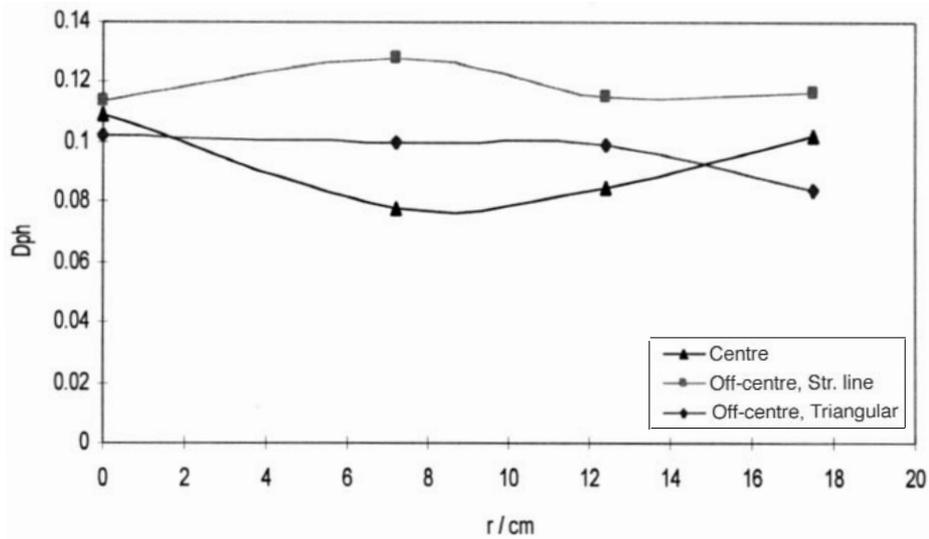
Figure 5. Effect of tuyere configuration on the radial variation of the Dph on the left-axis of the tank ( $0.00599 \text{ m}^3/\text{s}$  and  $z = 5 \text{ cm}$ )
