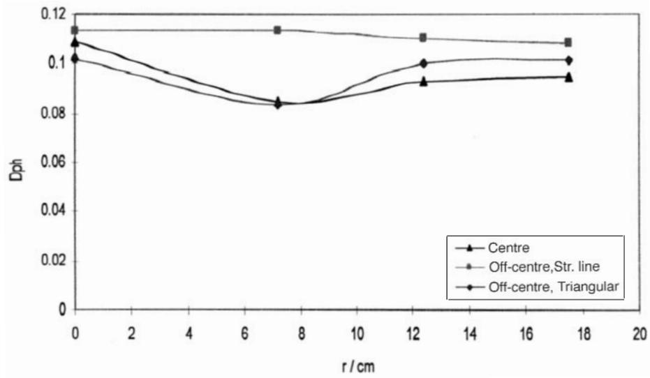
Figure 8. Effect of tuylene configuration on the radial variation of the Dph on the right-axis of the tank (0.00599 m<sup>3</sup>/s and z = 5 cm)
