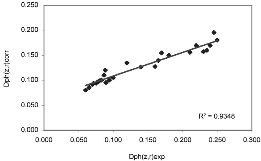
Figure 12. Comparison between the experimental and calculated values of the dispersed phase holdup
