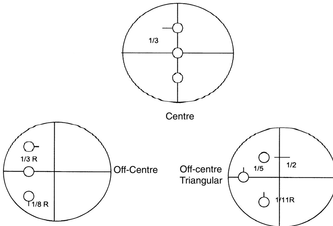
Figure 1. Tuyere configurations used in the present study
