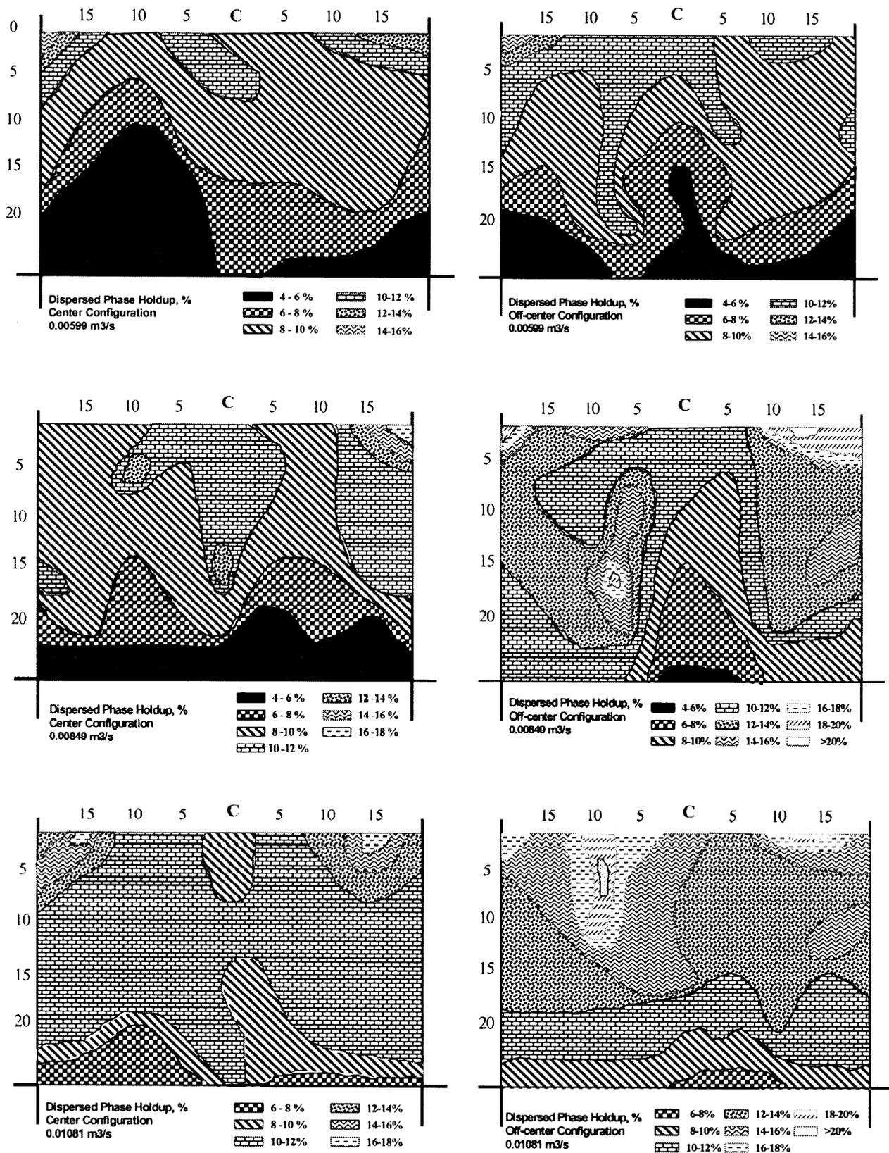
Figure 11. Comparison of dispersed slag phase holdup between off-centre straight and centre configuration along the left-right axis
