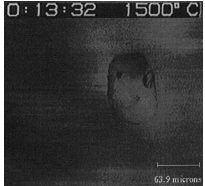
Figure 2. A typical example of an image obtained from the LSCM showing an alumina particle in a CaO-SiO 2 -Al 2 O 3 slag
