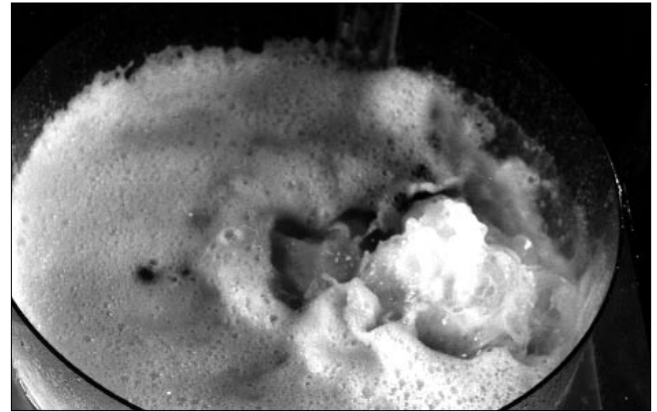
Figure 7. Top view of surface of the 3D model for slag/metal simulation, using zinc chloride-silicone oil
