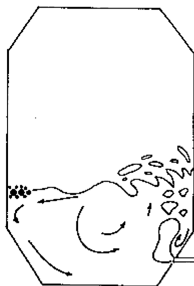
Figure 4. Schematic of induced fluid flows and mixing behaviour of simulated ferro-silicon granules and lumps in the slice 2D model in the absence of a slag phase
