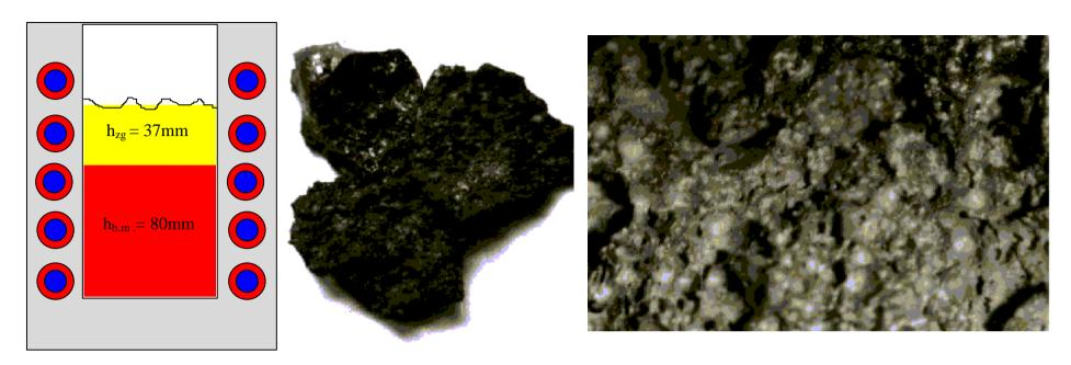
Steel: C = 0.2%; Natural size X 10 Microscopic slag aspect Macroscopic slag aspect quantity = 2 kg;Slag: **RESULTS** CaO = 50%;  $SiO_2 = 25\%$ ; m = 1,6626g $V_a = 1.5 \text{ cm}^3$ ;  $\rho_a = 1.1084 \text{ g/cm}^3$ ; FeO = 25%;  $V_s = 0.8 \text{ cm}^3$ ;  $\rho_s = 2.0782 \text{ g/cm}^3$ ;  $I_B = 2;$ quantity = 0.2 kg; holes percentage = 46,66%; C = 25%**Micropellets**: Porous material with uniform porosity ( $\phi_{\text{bubbles}} = 0.5 \div 2 \text{mm}$ ), Fe = 45%Ca = 15%
