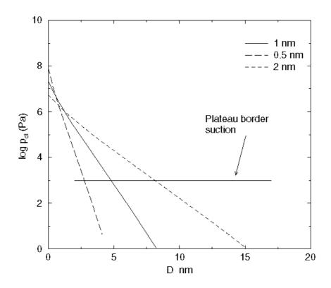
Figure 6 Calculated force of repulsion between two double layers of a thin film of thickness D. ( $\mathbf{Y}_0 = 0.275 \text{ V}$ )
