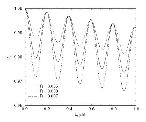
Figure 5 Plots of relative intensity versus thickness showing the effect of R.
