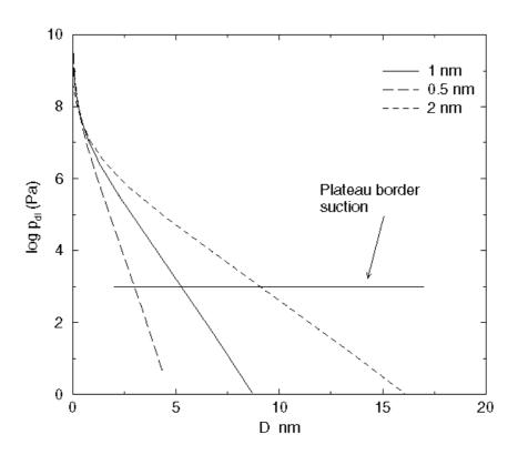
Figure 7 Calculated force of repulsion between two double layers of a thin film of thickness D. ( $\mathbf{Y}_0 = 0.55 \text{ V}$ )
