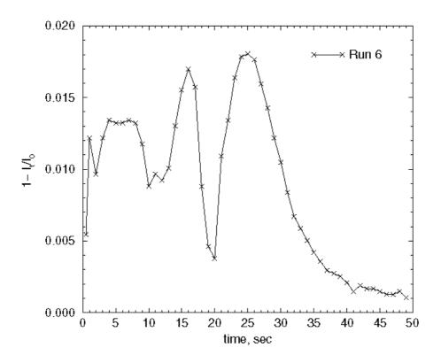
Figure 1 A typical relative intensity curve of the absorption of a laser beam through a liquid film of slag of 1.3%  $P_2O_5$ , 15%  $Al_2O_3$ , 9.6%  $Fe_2O_3$  with  $CaO/SiO_2=0.6$  at 1573K.
