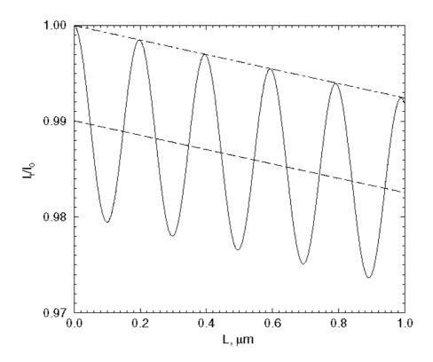
Figure 3 Plots illustrating the relative intensity of the transmitted laser beam through thin films ( $a = 7.6 \text{ mm}^{-1}$ ). Solid curve: coherent beam transmission; dashed line: incoherent beam transmission; dot-dashed line: Lambert's law limit (incoherent beam and no reflection).
