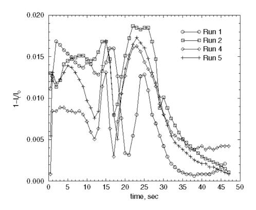
Figure 2 Results of the repeated measurements of the relative intensity curve of the absorption of a laser beam through a liquid film of slag of 1.3%  $P_2O_5$ , 15%  $Al_2O_3$ , 9.6%  $Fe_2O_3$  with  $CaO/SiO_2=0.6$  at 1573K.
