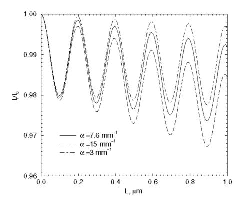
Figure 4 Plots of relative intensity versus thickness showing the effect of a.
