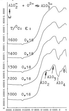
silicate melts). In solid silicates(1000-1200°C) WAVENUMBERS (CM-1) the transformation of the glassy in the crystallized(Wollastonite,Diopside) state (time dependnce) was measured by IR-emission. To obtain the accurate position of the emission maxima and the intensities we carried out curve-fittings by using gaussian functions. The present investigations deal with the solution of gases (H2O in CaO-Al2O3 and H2O/HF in CaF2-CaO-Al2O3, method in [1]) in the slags.
