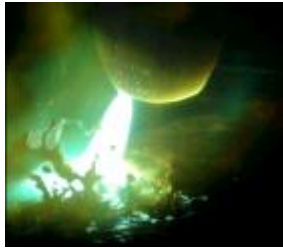
Fig.8 Violent splashing at 2 kA
