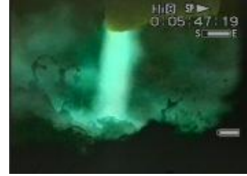
Fig.9 Thicker arc with splashing at 8.1 kA (Image L16354)
