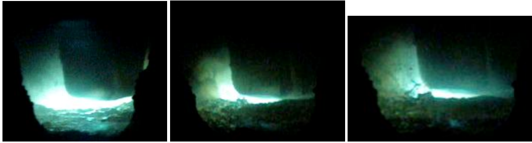
Fig.16 Industrial steelmaking arc at 40 kA, 450 V (full power is at 70 kA, 550 V)
