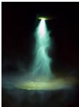
Fig.5 Arc about to become unstable
