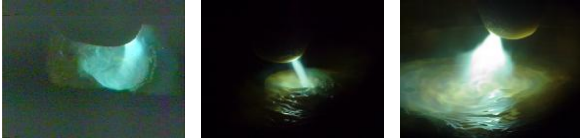
Fig.14 Arc depressions – punched hole and smeared depression (Images C0833, FL025, FL028)
