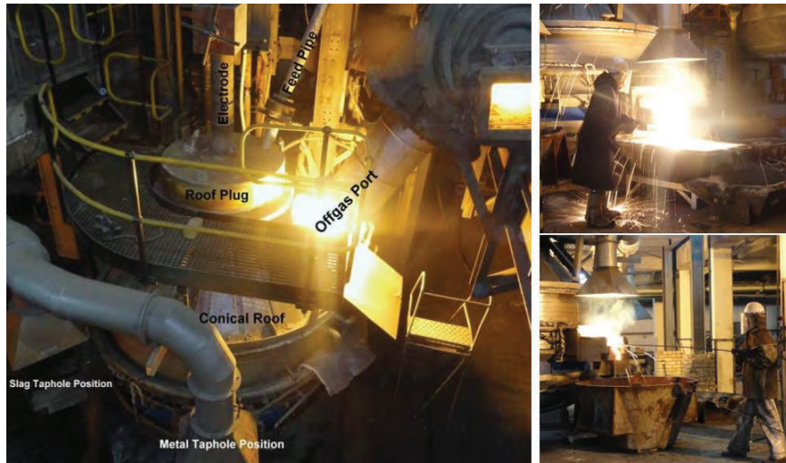
Figure 3. View of the pilot furnace in operation (left) - annotations indicate relevant aspects of the furnace, and a metal and slag tap in progress (top and bottom right), photographs by author
