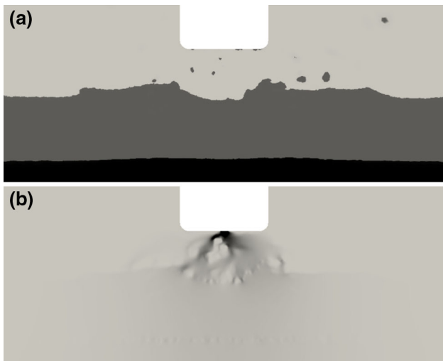
Fig. 8. (a) phase field and (b) current density field at 570 ms, 5-cm arc length, and 1-kA current.
