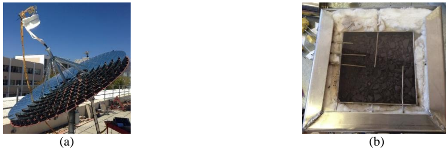
FIGURE 1. The experimental set-up showing the concentrator (a) and the box containing the ore sample (b).
