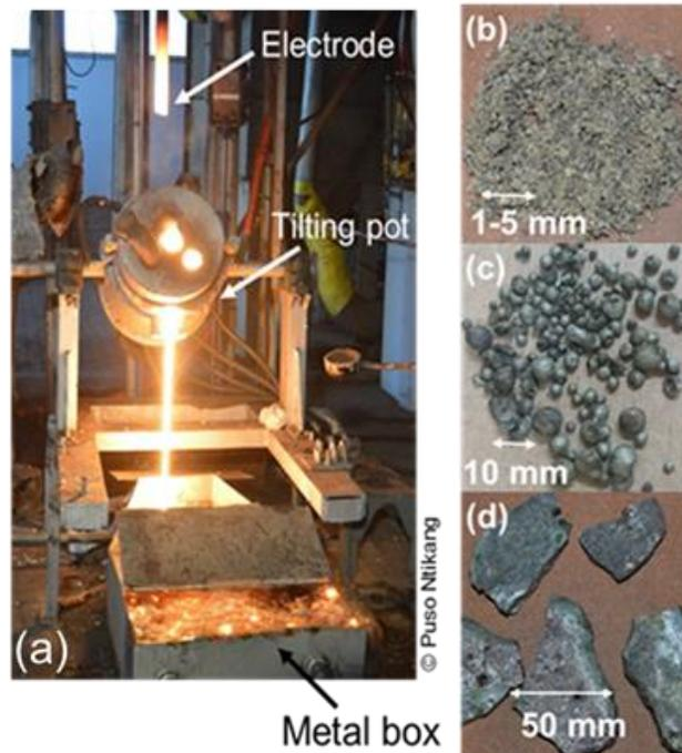
**Figure 1:** (a) 40 kW DC “tilting” pot facility, (b) Granulated slag product, (c) entrained SiMn product, (d) SiMn alloy product
