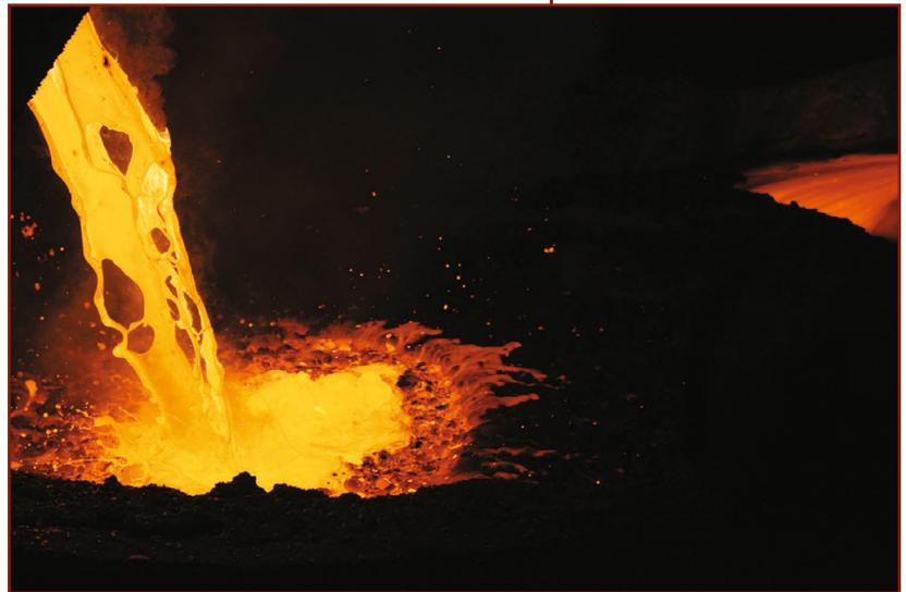
**Follow Me:** Liquid silicomanganese alloy and slag flowing from the tap launder into the metal ladle, and then slag into the slag pot, Transalloys, South Africa, March 14, 2013 © Joalet Steenkamp.
