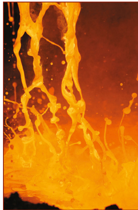
Dance: Liquid silicomanganese alloy and slag flowing into the ladle at Transalloys, South Africa, March 14th, 2013 © Joalet Steenkamp.
