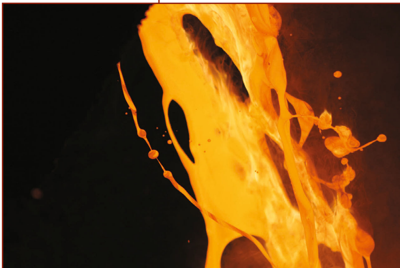
Sphere: Liquid silicomanganese alloy and slag tapped from a sub-merged arc furnace at Transalloys, South Africa, March 14, 2013 © Joalet Steenkamp. This image is now on permanent display at TMS headquarters.
