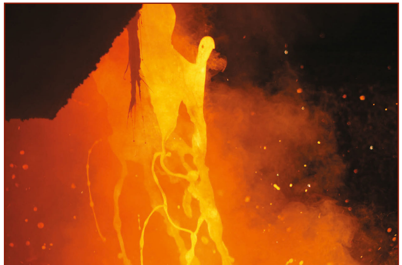
Beard on Fire: Liquid silicomanganese alloy and slag flowing from the tap launder to the ladle at Transalloys, South Africa, March 14th, 2013 © Joalet Steenkamp.
