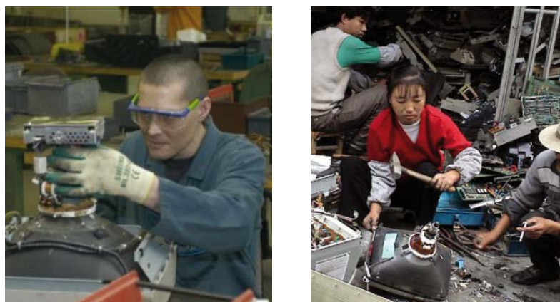
Figure 2: CTR removal in the dismantling step: safe practice in Switzerland (left), hazardous practice in China (right)
