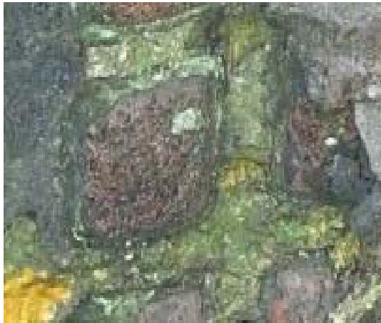
Figure 6. Typical corroded cooler – yellow elemental sulphur deposited on black copper sulfide corrosion product on copper. Grey covering is frozen slag accretion
