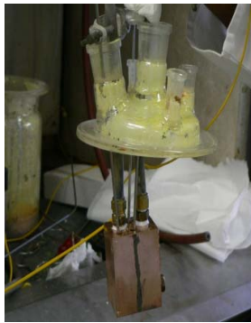
Figure 10. Suspended water-cooled copper test piece before insertion into test rig
