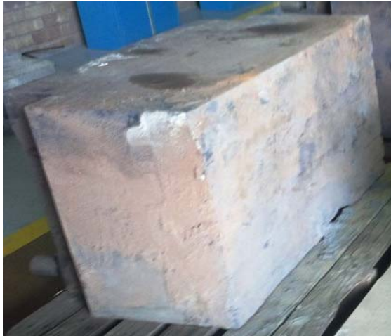
Figure 18. Upper cooler copper and graphite in pristine condition after being installed in the furnace for 12 months
