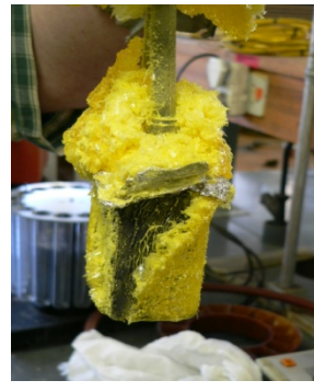
Figure 12. Water-cooled copper specimen coated with sulphur after testing
