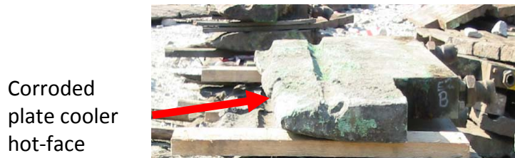
Figure 4. Severe upper plate cooler corrosion at Waterval Smelter. Note increased corrosion of upper plate cooler located in the furnace nearest the top of slag and concentrate interface
