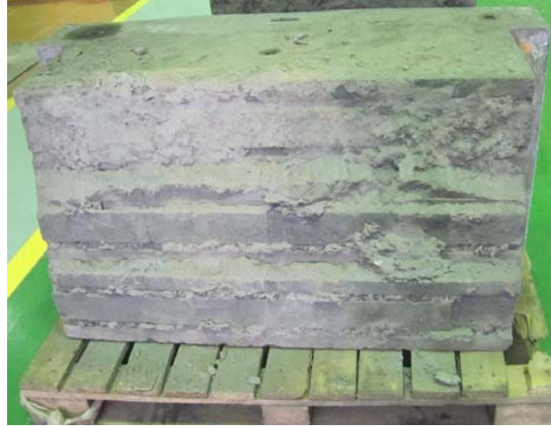
Figure 19. Perfect lower cooler graphite hot-face after being installed in the furnace for 12 months
