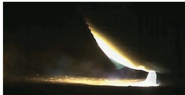
Figure 4—Arc at anode electrode, 3 kA, 15 mm arc length, 200 mm electrode
