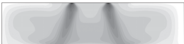
Figure 7—Projected temperature field, 0.04 m separation, 50 mm arc length
