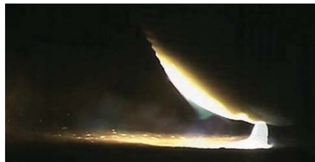
Figure 5—Arc at anode electrode, 3 kA, 15 mm arc length, 200 mm electrode
