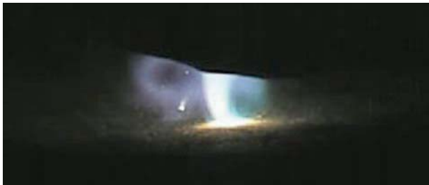
Figure 2—Arc at anode electrode, 1 kA, 20 mm arc length, 200 mm electrode
