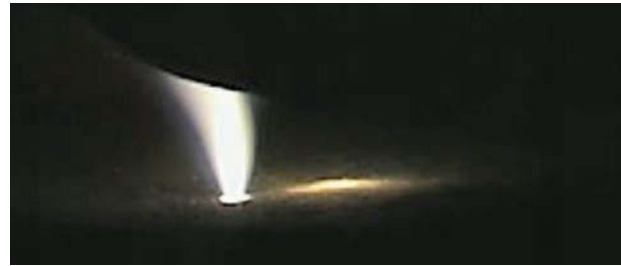
Figure 3—Arc at anode electrode, 1 kA, 20 mm arc length, 200 mm electrode
