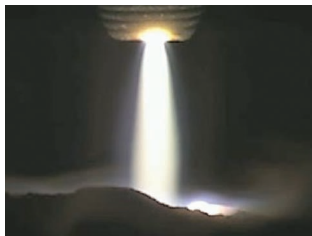
Figure 4—Cylindrical, steady-state arc in air at 500 A, 5 cm arc length
