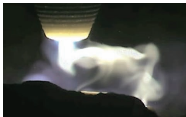
Figure 6—Chaotic arc at 2000 A, 5 cm arc length
