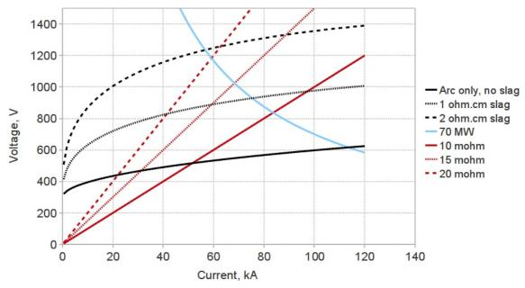
**Figure 12:** The relationship between voltage and current for an industrial-sized furnace operating at a fixed arc length of 50 cm and with a slag depth of 60 cm (for an arc resistivity of  $0.0175 \ \Omega cm$ )
