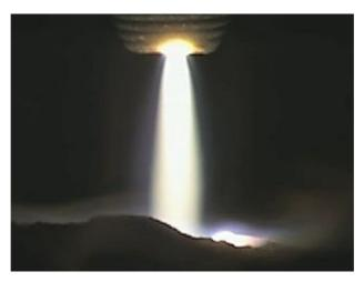
Figure 4: Cylindrical, steady-state arc in air at 500 A, 5 cm arc length
