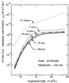
**Figure 8**: Volumetric radiation emission, assuming black body radiation
