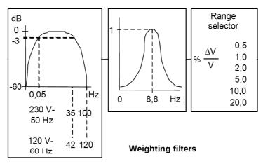
Figure 14: The norm DIN EN 61000-4-15 specifies how to measure flicker
