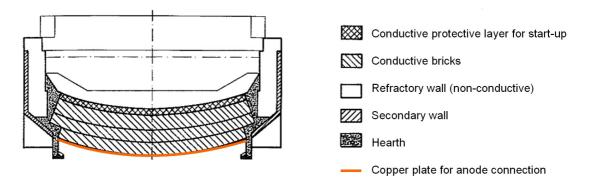
Figure 15: Principle sketch for conductive bottom electrode
