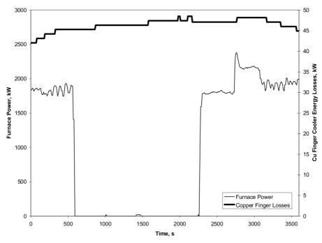
Figure 10: Measured transient energy losses from a copper finger cooler<sup>12</sup>
