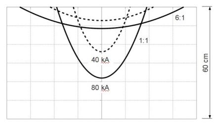
**Figure 11:** Dimensions of the cavity formed by arc jet thrust at different diameter: depth ratios, in the case of a current of 40 kA (dotted lines) or 80 kA (solid lines) and a slag density of 3500 kg/m3 and thickness of 60 cm
