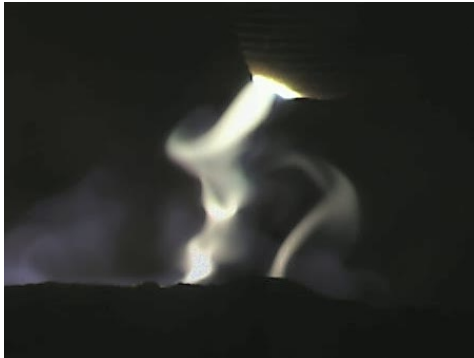
Fig. 6. Image of arc at 1000A and 10cm arc length, 5000 frames/s, shutter 4 ms, anode arc at lower right
