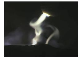
Fig. 6. Image of arc at 1000A and 10cm arc length, 5000 frames/s, shutter 4 ms, anode arc at lower right
