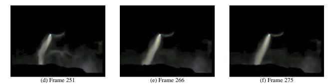
Fig. 8. Frames from a high-speed video sequence of an arc at 1000A and 10cm length, showing a temporary transition from irregular dynamics to a pseudo-stable arc column, 30 000 frames/s, shutter 4 µs
