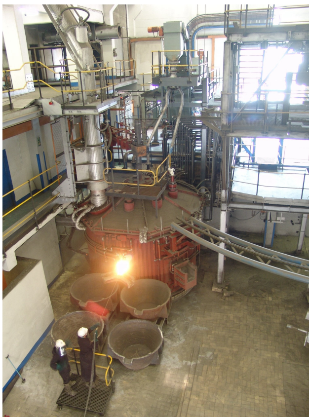
Figure 1 – First slag tap from Mintek's 3 MW furnace, 4 October 2008
