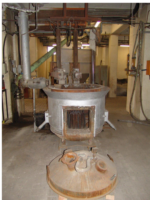
Figure 17: 200 kW furnace – either AC or DC, with 1, 2, or 3 electrodes
