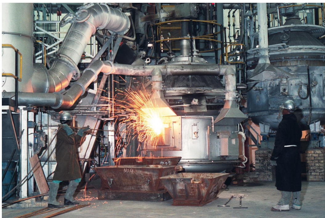
Figure 8: Ilmenite smelting testwork at Mintek
