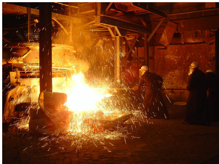
Figure 16: ConSmelt process – alloy being tapped
