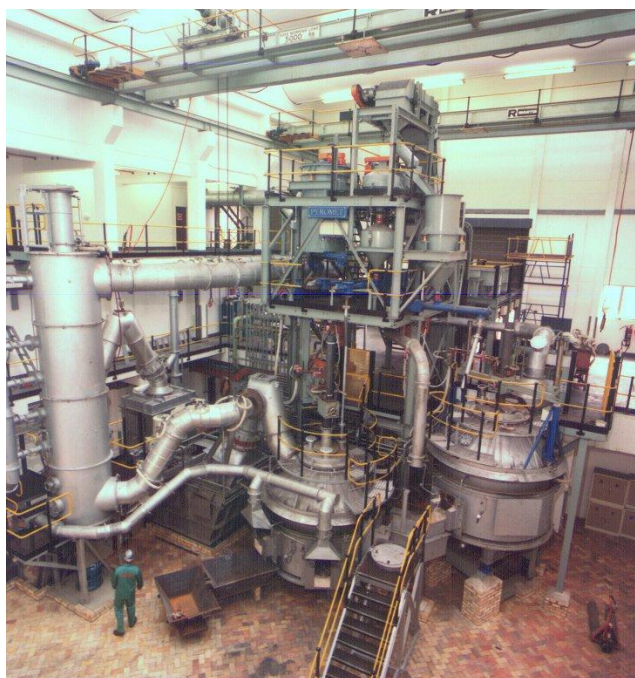
Figure 11: 5.6 MVA DC arc furnace pilot plant at Mintek (2 t/h pilot plant, including a zinc condenser, was commissioned in 1994)
