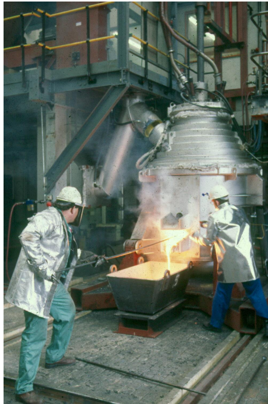
Figure 6: The 3.2 MVA DC arc furnace at Mintek being tapped
