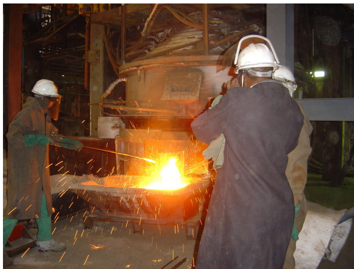
Figure 15: ConSmelt process – alloy being tapped
