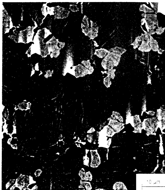
Fig. 6 — Back-scattered electron image of the magnesia-stabilized zirconia electrolyte supplied by Nippon Kagaku Togyo.
