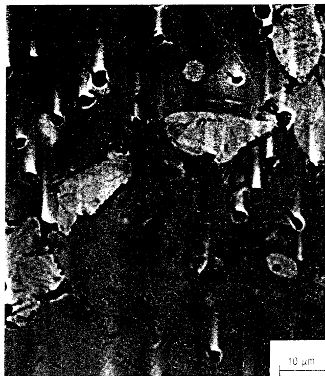
Fig. 7 — Back-scattered electron image of the magnesia-
