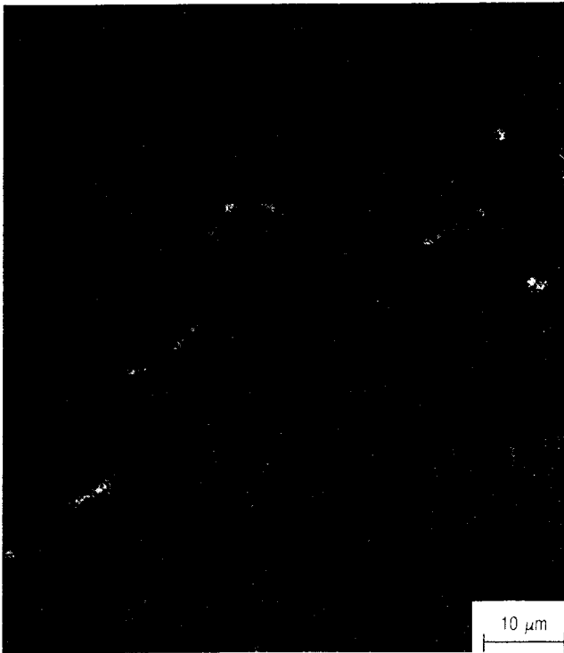
Fig. 9 — Characteristic X-ray image of the magnesia-stabilized zirconia electrolyte from Corning showing the distribution of magnesium.
