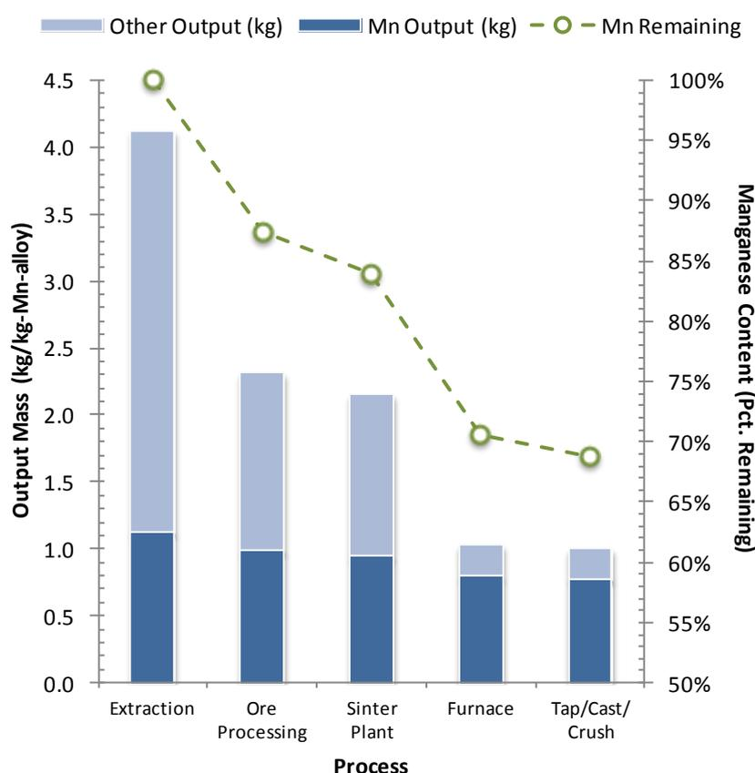
**Figure 14:** Manganese throughput and losses by supply chain stage for industry average ferromanganese production.
