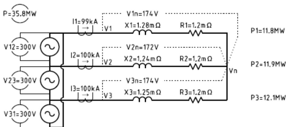
**Figure 8:** Simplified furnace circuit model with sample values
