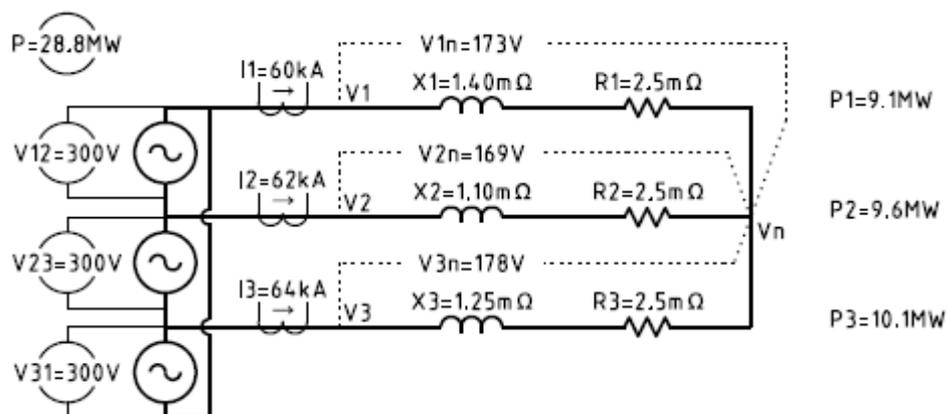
**Figure 10:** Circuit model with higher power factor
