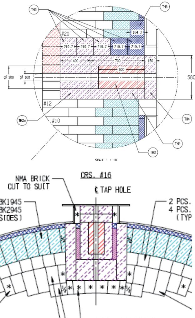
Figure 2: GrafTech improved tap hole configuration
