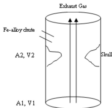
Figure 2: Higher speed of exhaust gas ( $V_2$ ) due to area ( $A$ ) effect
