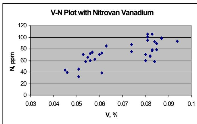
Figure 1: Nitrogen recovery for different levels of V in steel
