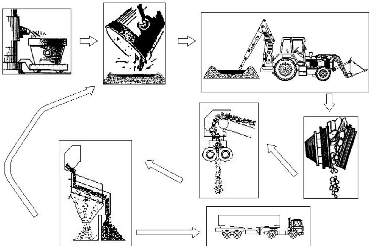
Figure 1. Conventional processing technology in a ferroalloys factory after metal tapping.
