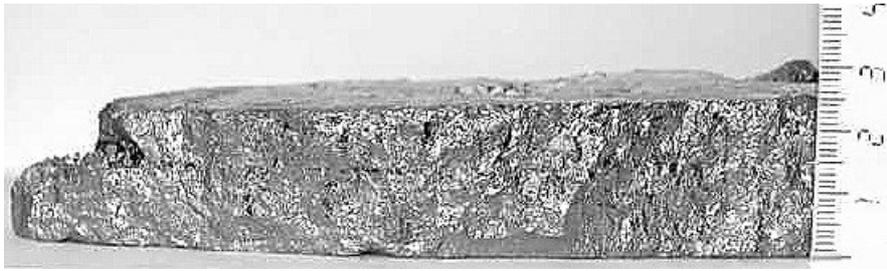
Figure 5. Thicker layer silicon cast onto the machine.
