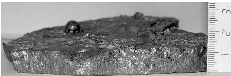
Figure 4. Thin layer silicon cast onto the machine.
