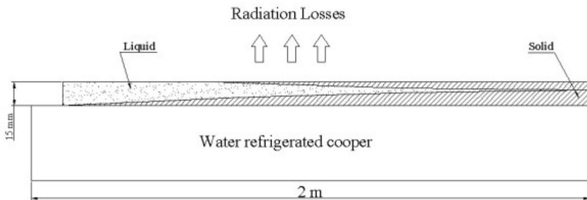
Figure 3. Schematic of silicon solidification on the water-cooled copper plate.
