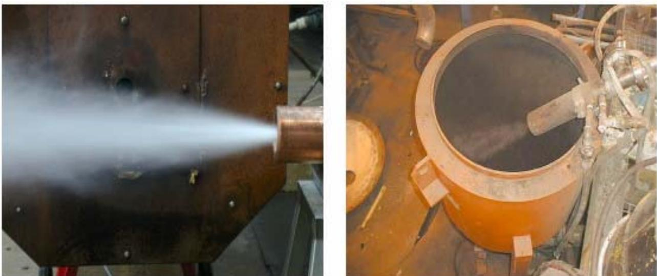
Figure 3. The photograph on the left shows atomization illustrated by water. On the right is the atomization of sludge, in this case blast furnace sludge containing 48% water.
