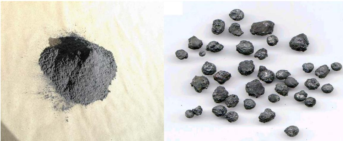
Figure 5. The processing of dust with oxyfuel technology, “before and after” photographs. Here, ferrochromium dust at  $-0.1$  mm (left) is recycled and turned into virtually all-metallic agglomerates of 3-8 mm.
