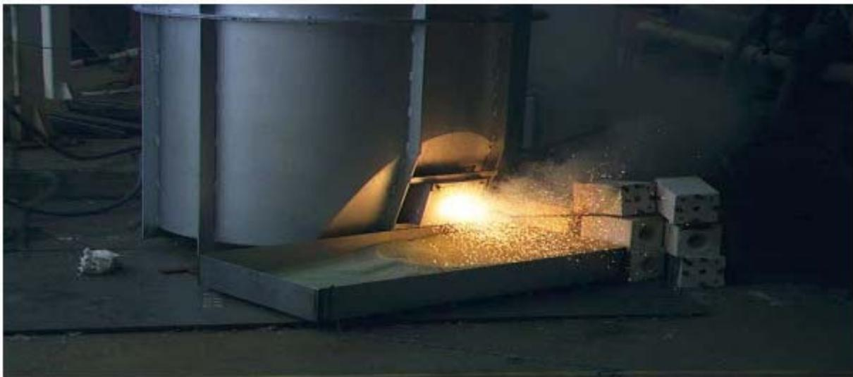
Figure 4. Photograph taken during the first pilot-scale trials with processing of ferrosilicon fines and dust. Here, a blend of liquid product and agglomerates is coming out of the taphole.
