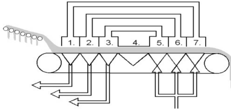
Figure 1. Steel belt sintering process. 1. Drying section, 2. Heating section, 3. Sintering section, 4. Balancing section, 5., 6. and 7. Cooling sections.
