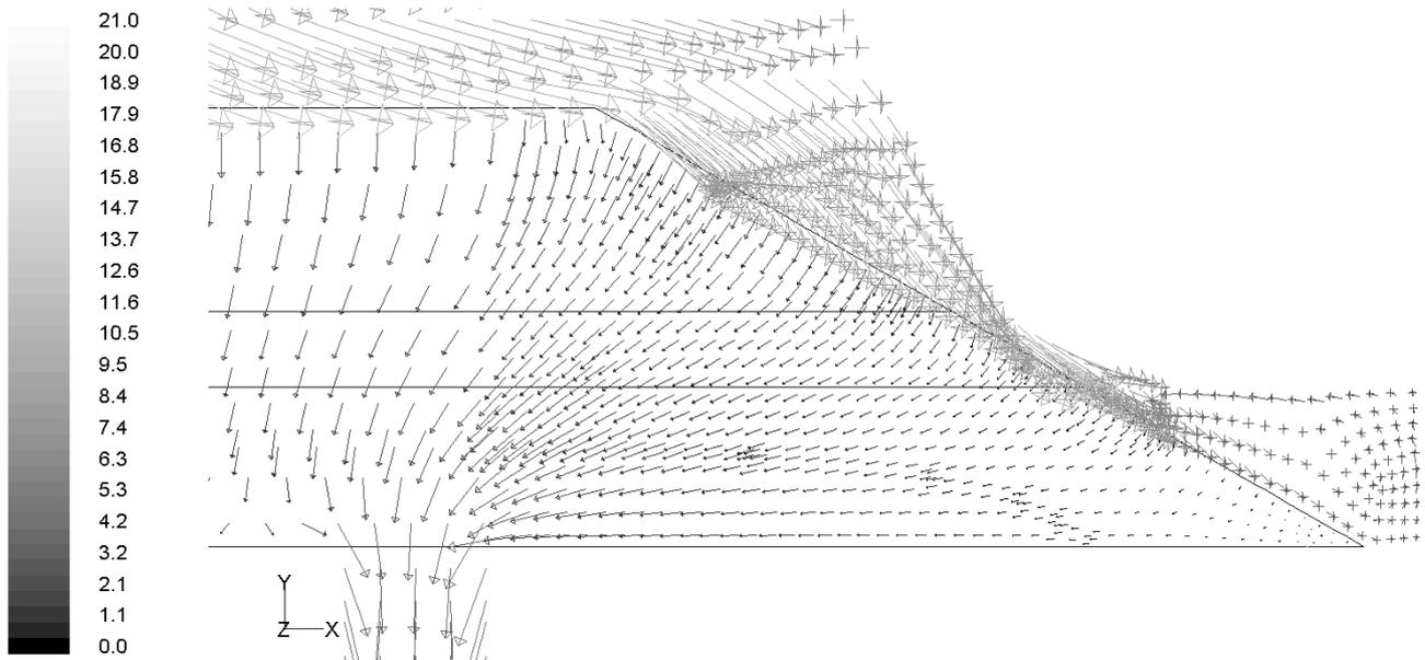
Figure 8. Velocity vectors of the gas in the drying compartment. A detail from the side of the bed on a plane the across the bed.
