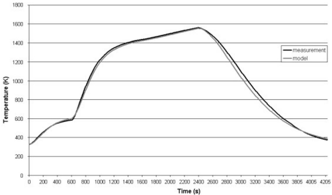
Figure 4. Comparison between measured and modelled gas temperature in batch sintering experiment with chemically inert and dry pellets.
