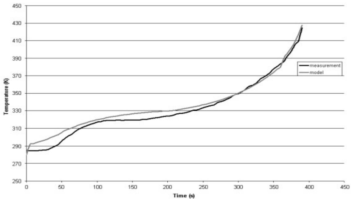
Figure 5. Comparison between measured and modelled gas temperature in batch sintering experiment in the drying compartment.
