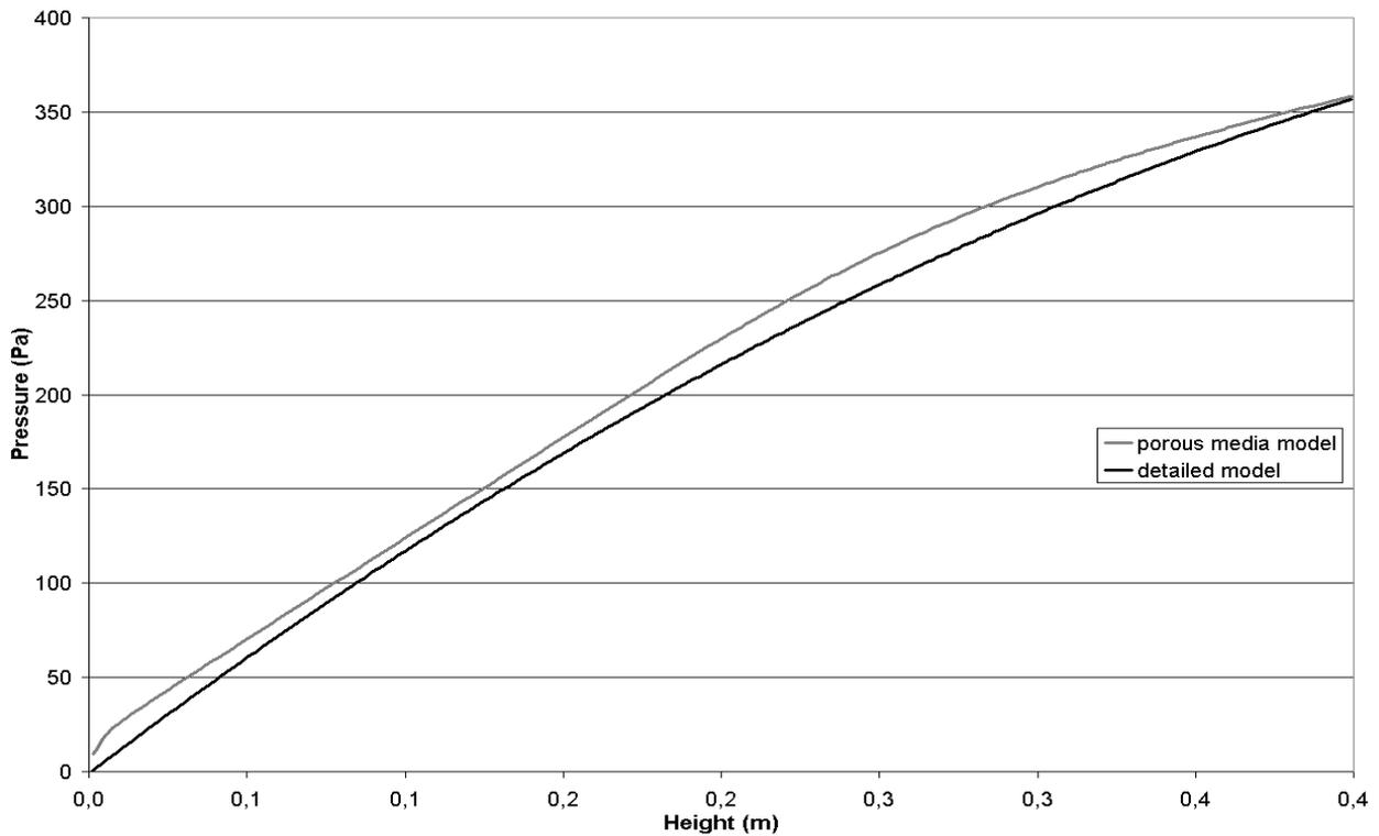
Figure 2. The comparison of the pressure drop inside a sintering bed when detailed and porous media models are used.
