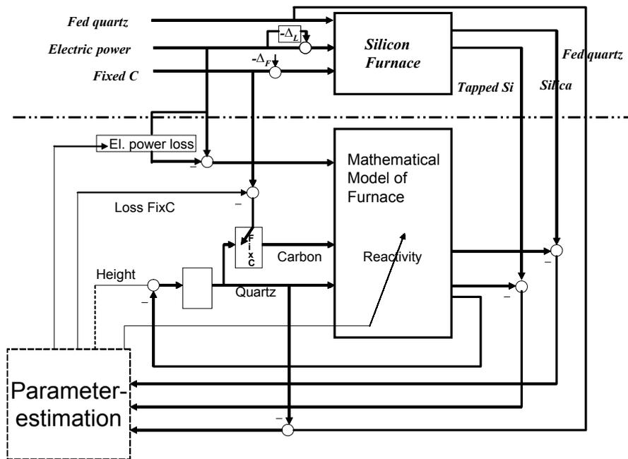
Figure 2. Overall concept for parameter estimation.
