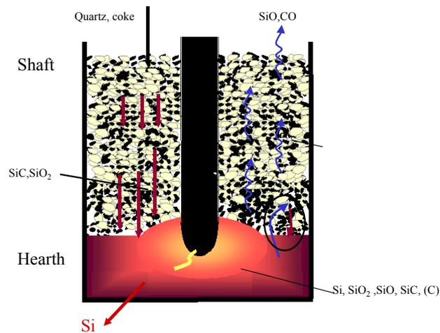
Figure 1. Mass transport in the Silicon furnace.
