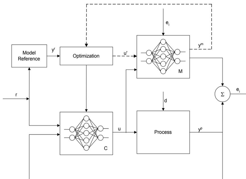
Figure 5. Model predictive control structure using neural networks [21].
